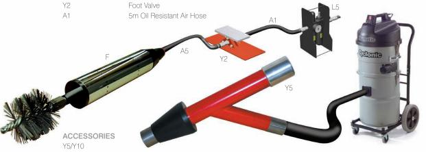
Vacuum Attachment (Y Piece) - this unit is invaluable to the cleanliness of the boiler or the area being cleaned as it is the link between the tool and the vacuum unit. As the tool is removed on it's return to the operator, all the debris that has collected in the tube is sucked in to the vacuum via this unit.
